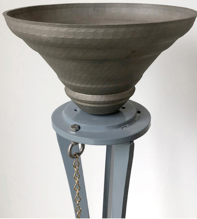
3D Printed Difference Tone Bell 2017. 3D print in 316 stainless steel/tin bronze by Exone in the USA. Dimensions: 1150mm high x 470mm diameter
